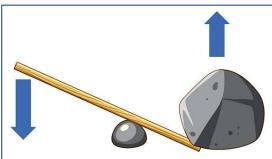
Pushing on the long end of a **lever** reduces the effort needed to lift the load.
